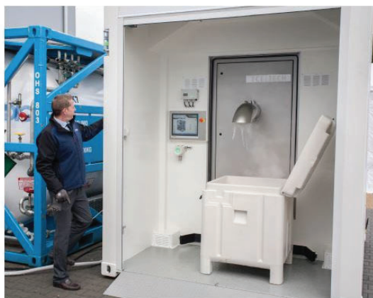
Dry Ice Production Hub up to 120 kg/hr | 265 lbs/hr OR up to 350 kg/hr | 772 lbs/hr
