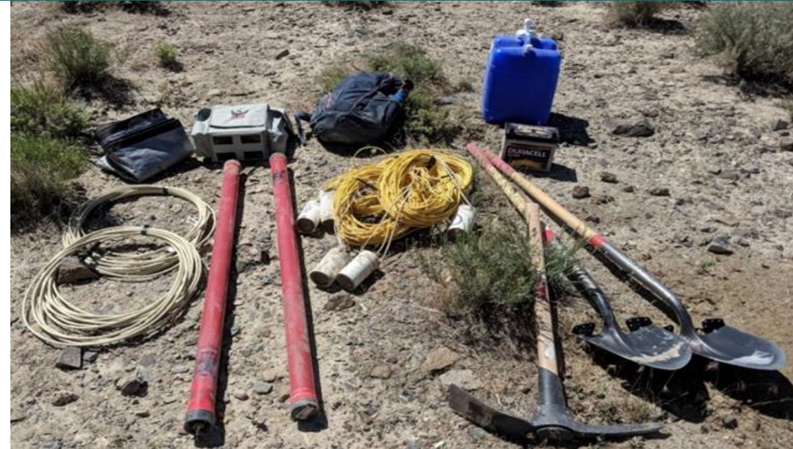
Induction coils (red tubes), Telluric sensors ‘pots’ (white cylinders), Data logger & GPS (grey case). Cables, battery, water and shovels.
