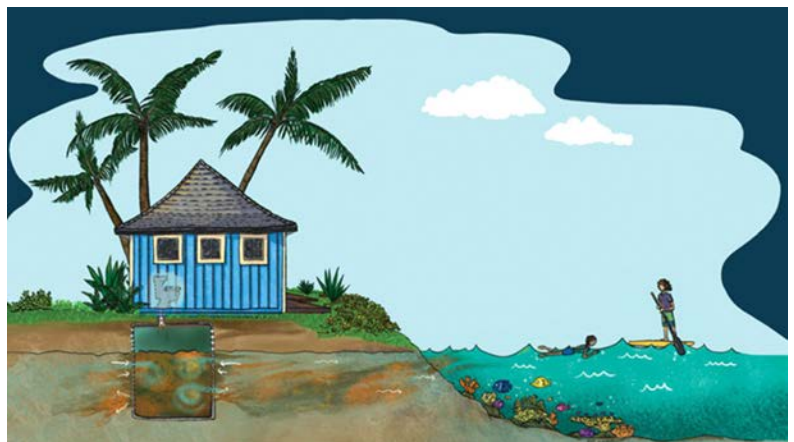
Image of how a cesspool contaminates groundwater and marine resources. Untreated human waste flows from open spaces in the cesspool to groundwater which eventually connects to seeps in the ocean potentially transferring pathogens and nutrients to reefs. Source: Elle Wibisono; Ka Pili Kai.
