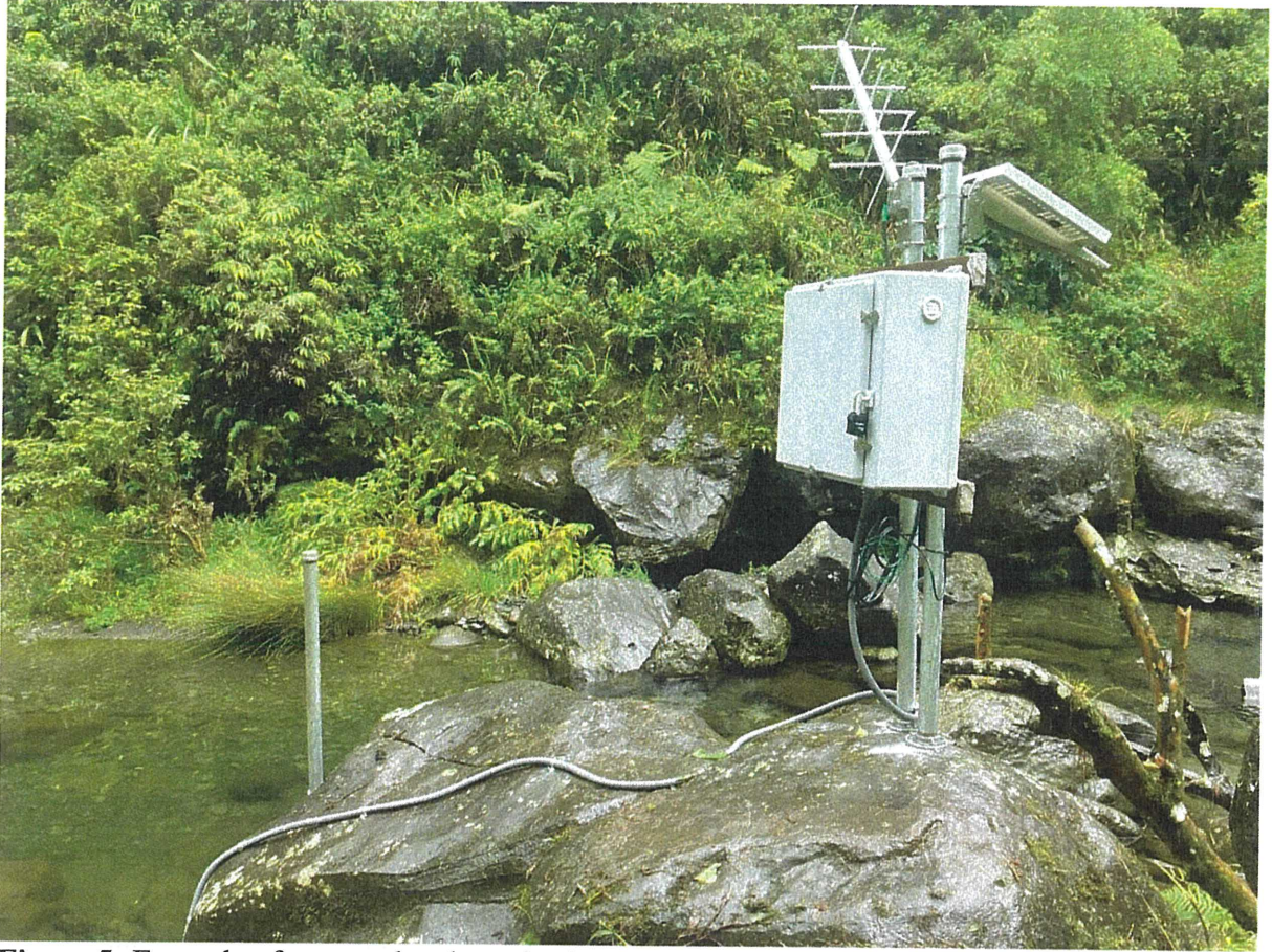
Figure 5: Example of a water-level monitoring station equipment mounted to steel pipes and flange mounted into rock.
