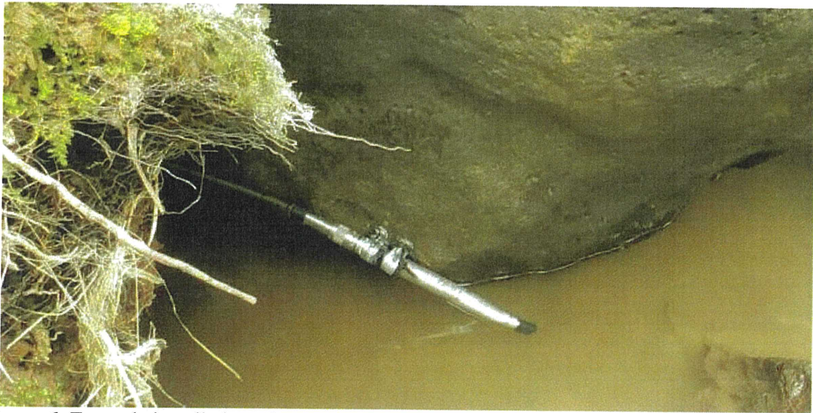
Figure 6: Example installation of stage sensor attached to bedrock with anchor bolts.
