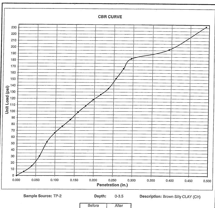
Relative Compaction (%): Moisture Content (%): Dry Density (pcf): Percent Swell or Expansion Value (%): Compaction Test Method: CBR Value @ 0.1" Corrected: CBR Value @ 0.2" Corrected:
