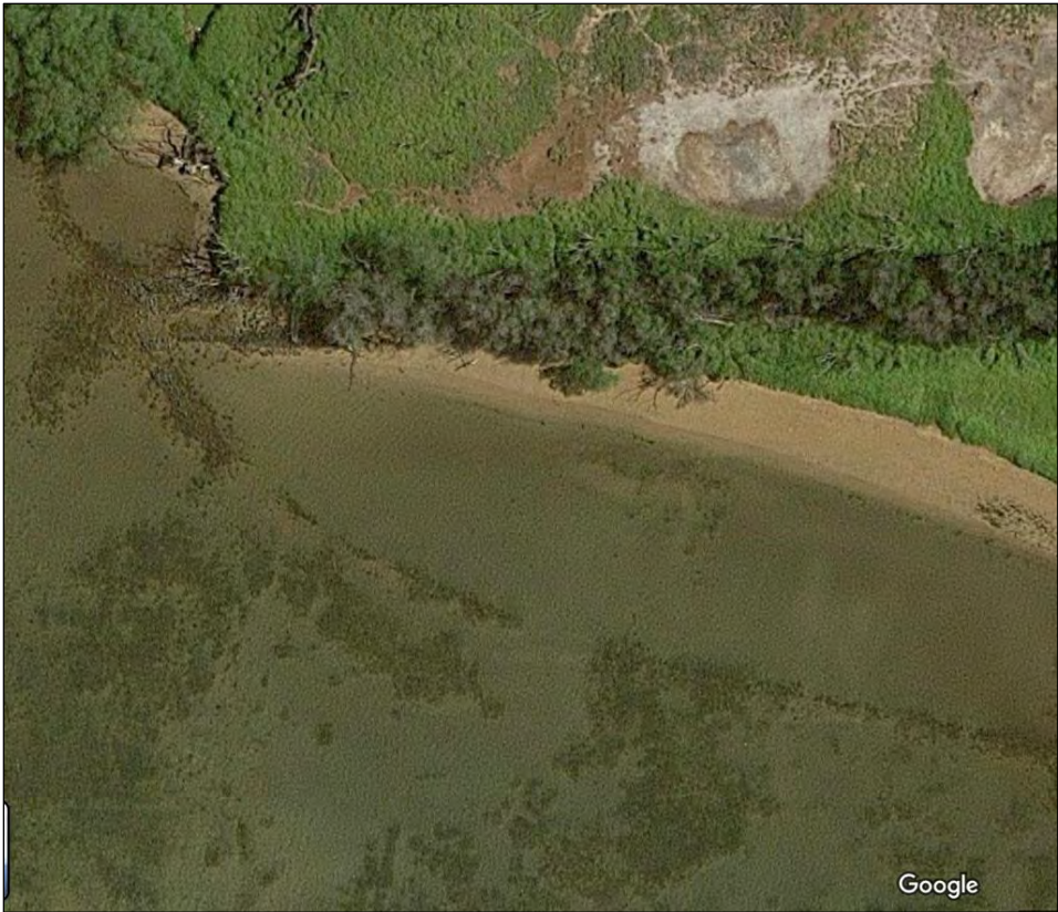
Photo: A remnant fishpond wall east of Kapa’akea acts as a sill to break wave energy thereby facilitating a beach corridor to form.
