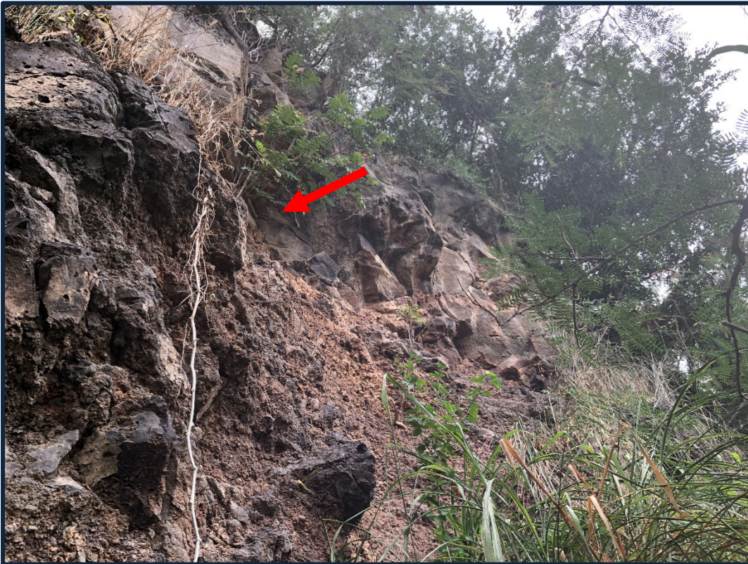
Photo No. 14 (TMK: 2-4-42: 17) – Possible source for 5-foot diameter boulder, located approximately 15 to 20 feet above the toe of the slope. Woody branch growing through rock face in this location; vegetation could have loosened large boulder.
