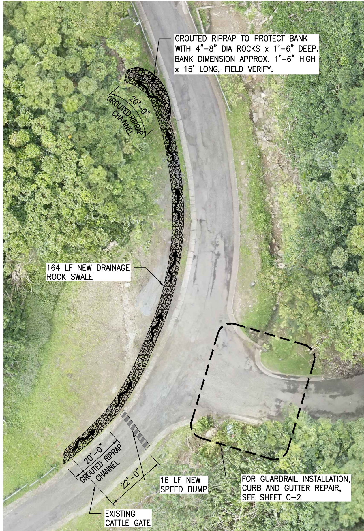
DRAINAGE SWALE PLAN SCALE: 1" = 20'-0"
