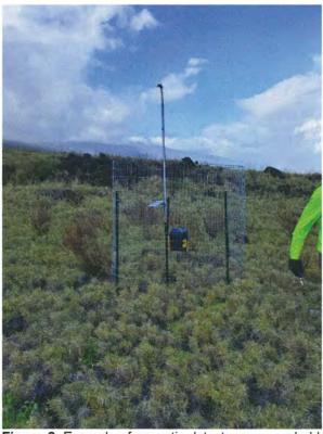
Figure 2. Example of acoustic detector, surrounded by 4ft enclosure fence, used in the 'Ope'ape'a (Hawaiian hoary bat) study.
