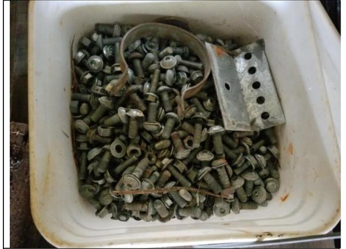
Tank Bolts – may need to be replaced?/ washers have a rubber gasket that maynot be 'good'
