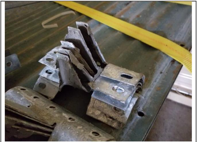
Tank Rib Clips est 36 each – Might need to be replaced due to excessive glue and some are damaged
