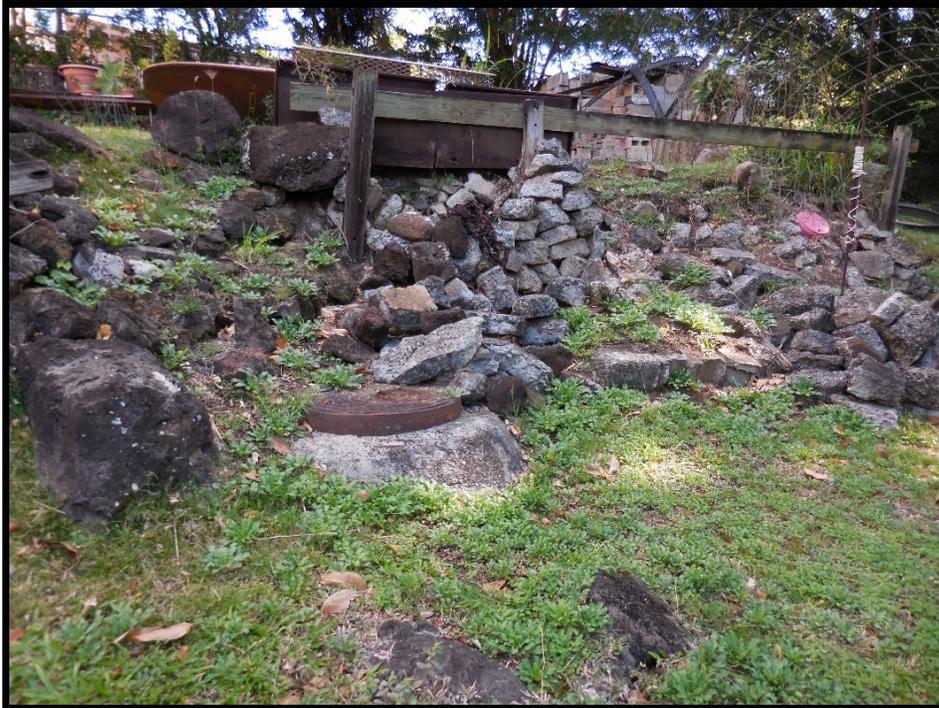
**Photograph No. 21:** Existing site condition at TMK: 1-2-4-042: 046 where a segment of existing pipe is planned for replacement by trenching. Note the ground surface soil condition with embedded hard basaltic boulders and surface boulder stockpiles. View is towards the northeast from the existing backyard manhole location. (dscn1949)
